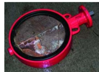
Picture 3: Severe galvanic corrosion of cast iron butterfly valve due to ground-contact with noble seawater cooler.
