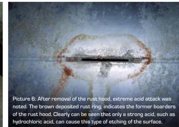
Picture 6: After removal of the rust hood, extreme acid attack was noted. The brown deposited rust ring, indicates the former borders of the rust hood. Clearly can be seen that only a strong acid, such as hydrochloric acid, can cause this type of etching of the surface.
