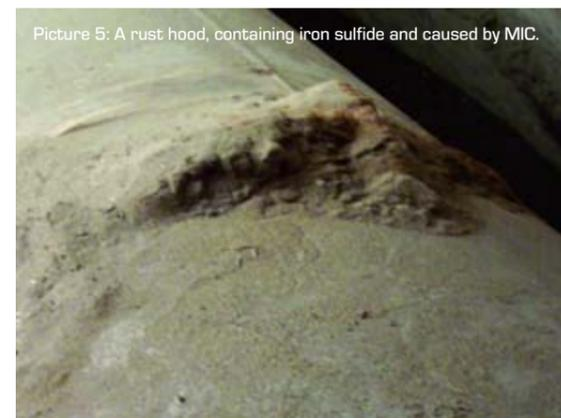
Picture 5: A rust hood, containing iron sulfide and caused by MIC.
