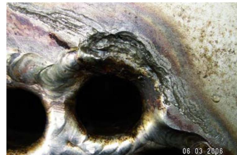
Picture 1: Crevice corrosion in seawater cooler. This corrosion finally leads to leakages.
